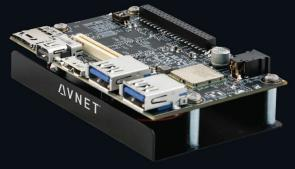
Ultra96<sup>™</sup> is an Arm-based, Xilinx Zynq UltraScale+<sup>™</sup> MPSoC development board based on the Linaro 96Boards specification.
