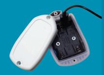
The Things Node is the perfect LoRa node to start prototyping your ideas without having to deal with bread boards, wires and sensors.
