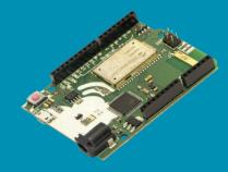
The Things Uno is the perfect board to start prototyping your IoT ideas or make an existing project wireless with up to 10km range by simply swapping boards.
