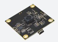
${\sf CAM8200-U}$  is a 5-megapixel USB digital camera module designed by Embest Technology.
