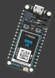
A powerful LTE CAT-M1/NB1 enabled development kit that can act as either a standalone cellular endpoint or LTE/3G/2G enabled gateway for Particle Mesh networks.
